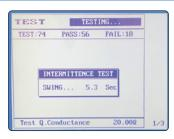
The Intermittence test function is swing test. Setting test time in seconds, the cable tester will continuously scan within the set time to perform a short-circuit judgment test.
