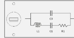
Most piezoelectric component connect to a circuit.
