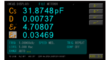
Monitoring \epsilon_r/\epsilon_r'' in Meter Mode
