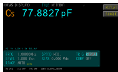
Apply DC Bias Voltage to Measure MOSFET Parasitic Capacitance
