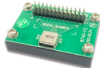
8740-F2 USB Type-C Test Fixture
